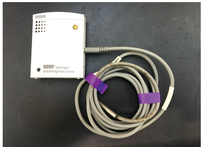
This is a simple data logger that will measure temperature and relative humidity. Data can be loaded by connecting the data logger to a computer and exporting it using the software that comes with the unit. Photos by Brian A. Krug.
